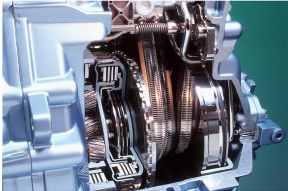
**The planetary gear set responsible for switching between forward and reverse gears is situated on the primary shaft of the Durashift CVT transmission (left), next to it the gear change clutch for the forward-rearward-shifting only and - more to the right - the pair of conical drive wheels for driving the power belt.**
