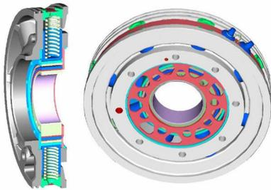
**The oil flow and pressure build-up of the radial piston pump have been custom tailored to the hydraulic supply requirements of the Ford Durashift CVT.**
