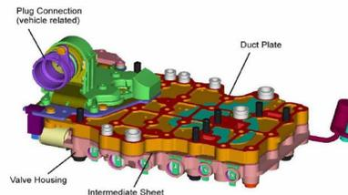
**The mechatronic module of the Durashift CVT packages all the control technology in a single control block. Also, there is no wiring harness inside the gearbox.**
