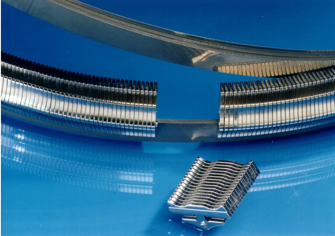
**The Van Doorne thrust link belt, shown here partially disassembled, consists of 400 links and two lines of steel belts with 12 rings each.**
