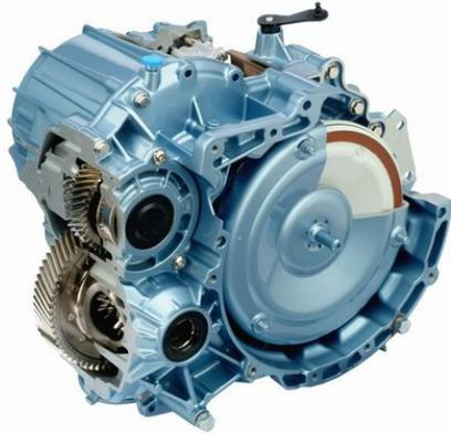
**On the drive side, the Durashift CVT transmission is equipped with a hydraulic torque converter, which, however is consequently bypassed by a clutch starting at very low engine speeds already.**
