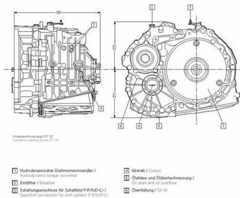
The Ford Durashift CVT's housing is a mere 381 millimetres long, making it ideal for use in front wheel drive vehicles.
