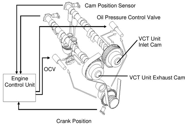
**The characteristic trait of the Ford Duratec Ti-VCT system is its fully variable control of both camshafts, driven by the parameters**
