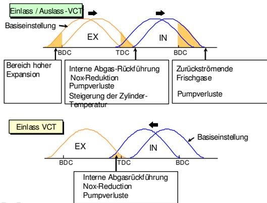
**Ford Duratec Ti-VCT also allows fine control over effects which may degrade the cylinder charge. Exhaust gas recirculation caused by larger overlap reduces nitrogen-oxides and improves fuel economy.**
