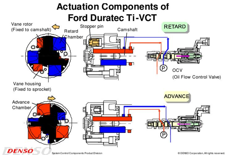
**Two variable control elements drive the rotation of the vane-type phase actuator fixed to each camshaft. The variable control is performed, powered only by the operating oil pressure of the engine, distributed via two 4.3-way valves.**
