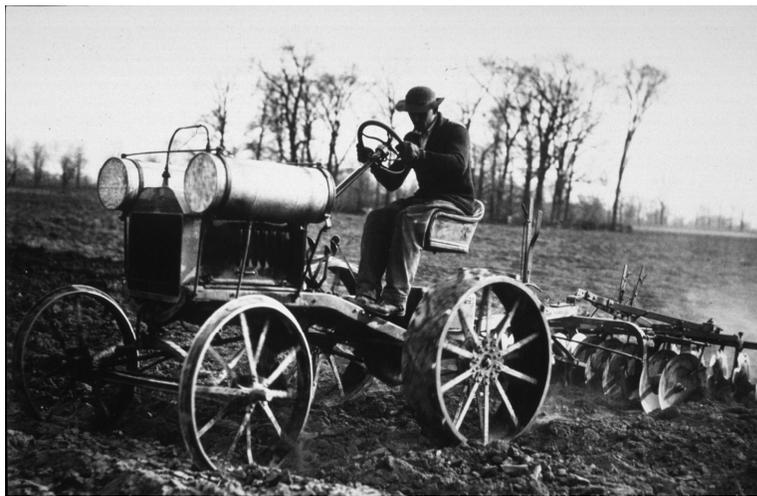
**In the good old days of Ford's Model T, engineers had not yet invented maximum engine speed. Instead, the engine's large cubic capacity was fully exploited to develop torque: "Tin Lizzy" delivered impressive 20 hp at 1800 rpm from its 2.89-litre displacement, and the veteran's maximum torque of 110 Nm at 900 rpm was not to be sneezed at either.**
