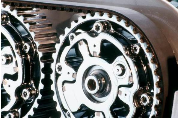
**Many active valve timing systems previously used were only able to vary timing between early and late. With its Duratec Ti-VCT system, Ford is now using the first map-controlled variable cam timing system in smaller engines: high-tech for better fuel economy and higher torque.**
