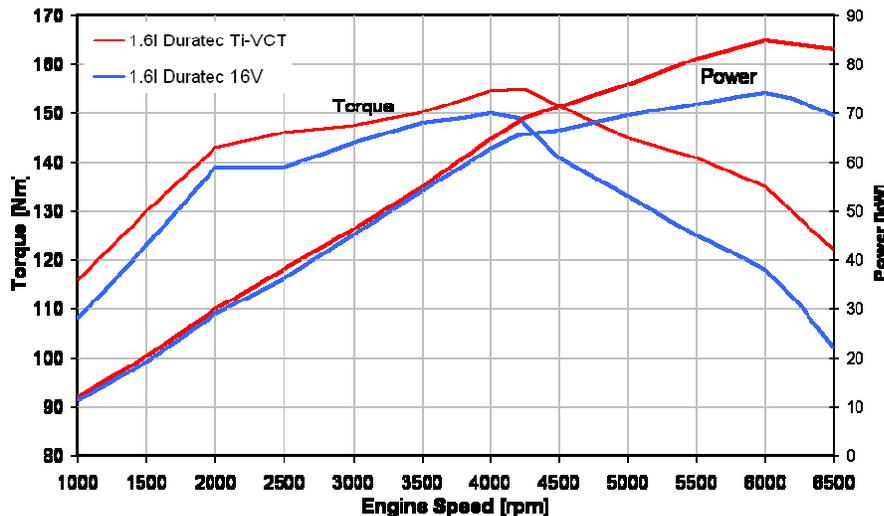
Ford Duratec 1.6 Ti-VCT shows an impressive torque curve over a wide range of engine speeds.
