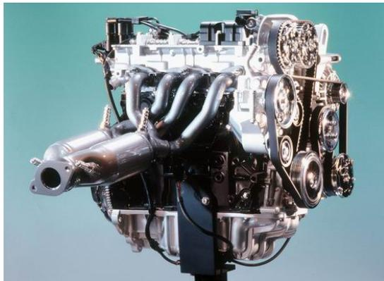
**The Ford Duratec Ti-VCT engine uses a double-flow catalytic converter. All of the mechanical components of this modern variable cam timing system are located inside the wheels driving the double overhead camshaft.**
