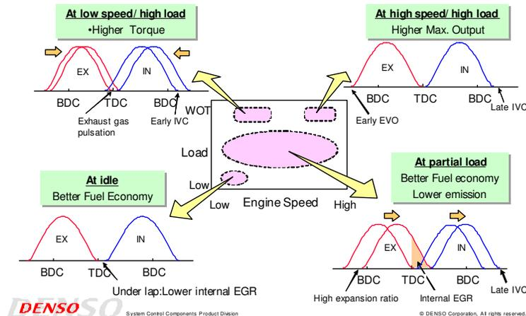
**In the medium engine speed and load range, timing is optimised to produce higher overlap. At idle and high engine speeds, these valve positions are avoided. Such sophisticated**
