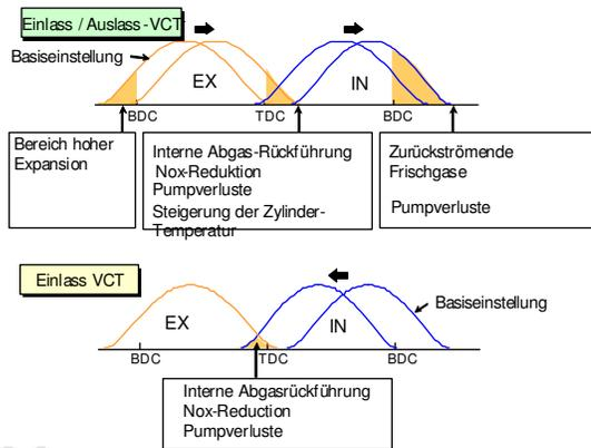
**Ford Duratec Ti-VCT also allows fine control over effects which may degrade the cylinder charge. Exhaust gas recirculation caused by larger overlap reduces nitrogen-oxides and improves fuel economy.**
